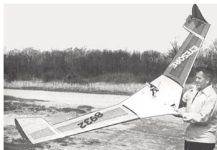
CF379 EYESORE. A 116" span R/C flying wing soarer with .19 eng. power pod. Plans on 2 sheets. D. McGovern. FM 8-75. $$J
