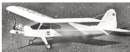
CF562 THE NEXT STEP. R/C trainer uses parts from ready to fly airplanes, or build it from plans. 36 span, .09 eng., 3 channel radio. B. Aberle. FM 3-81. $$C
