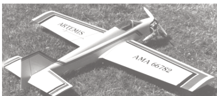
CF714 ARTEMIS. Aerobatic Sport-Pattern ship, featuring 58-inch span. .40 to .45 eng., 4 channel radio. R. Allison. FM 12-85. $$D
