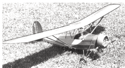
CF583 NICHOLAS BEASLEY NB-8. R/C Sport-Scale ship with 56-inch span parasol wing. For .09 eng., and 3 channel systems. A. Wolsky. FM 11-81. $$C
