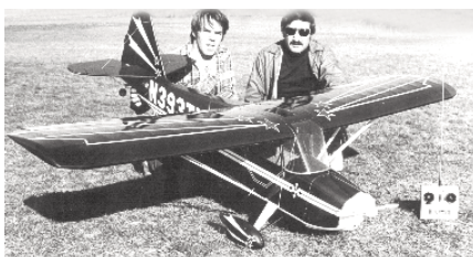
CF538 CITABRIA. Quarter-Scale R/C model of famous aerobatic trainer. For Quadra power, and 4 channel radios. Has 102-inch span. Plans on 2 sheets. T. Lombardo. FM 5-80. $$Q
