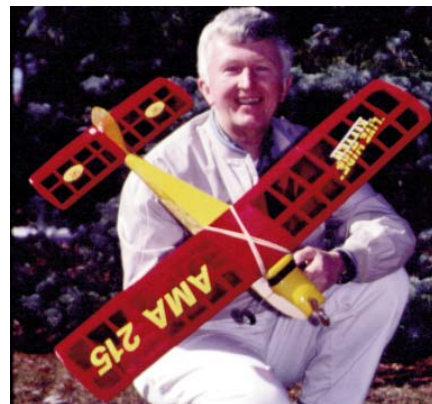
CF994 LIVE WIRE KITTEN. Electric powered replica of Hal DeBolt's 1950's design. 34-inch span, Speed 400 motor, Graupner 1:85:1 gearbox and 7 cells. 3 channel R/C. Aberle. FM 6-96. $$$C
