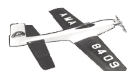
CF456 THE ACE THREE TEN. 3 channel R/C trainer, 36-inch span, .09 to .10 eng. B. Aberle. FM 12-77. $$$C
