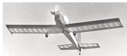
CF689 NACHO. R/C sportster, for .09 to .15 eng., has 44-inch span. For 3 to 4 channel gear. L. F. Randolph. FM 3-85. $$C
