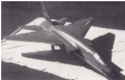
CD014 RA-5C VIGILANTE. Powered by a single Byro-jet with an O.S. .91 this plane builds from fiberglass and foam into a very easy flying scale "twin". Spans 63 inches, 87 inches nose to tail. Phil Knuckles. FM 1-97. $$$R
