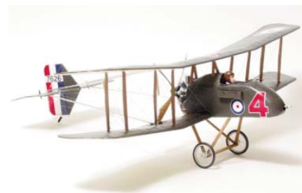
CD239 ROYAL AIRCRAFT FACTORY F.E.8 An R/C Scale Park Flyer of the famous WWI scout with a pusher engine. All balsa construction, with a wing span of 35 1/2 inches. Final weight is 6.5 ounces with a GWS IPS power system, 700 mAh 2-cell 5C Li-Po battery and 3 channel radio. Plans on one sheet. Hector Santemma. FM 12-2004 $$D
