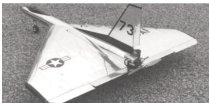
CF298 MOONROCK. Wild looking R/C Sport-Pattern delta with 44-inch span, and 46-inch length. For .45 eng., and 4 channel R/C units. L. Cubillos. FM 5-73. $$$
