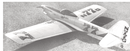
CF255 XP400. Formula II and FAI pylon racer with 56-inch span. Uses .40 eng., 4 channel R/C gear. D. Gierke. FM 3-72. $$D
