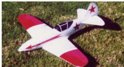
CD182 MIG-3 An R/C electric for AMA 704 Combat. Balsa and plywood construction, fully sheeted to take the beatings of landing without wheels. With a wing of just 30 1/2 inches, the finished weight is 16 ounces. Power is provided by a Speed 400 motor on a 7-cell pack. Plans on one sheet. Gus Morfis. FM 11-2002 $$C
