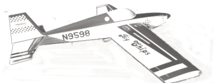
CF728 BIG CHIPS. R/C Sport design: two stroke .60, or 1.20 4-cycle eng. 71-inch span, 4 channel. L. Phillips. FM 7-86. $$F
