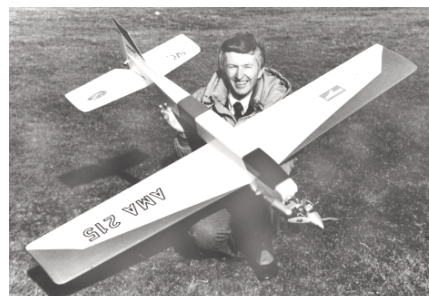
CF692 IMAGE. This practical R/C Sport-Pattern design features 72-inch span, and takes .60 eng. 4 channel gear. B. Aberle. FM 4-85. $$D
