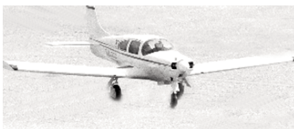
CF287 WINDECKER EAGLE. R/C Scale model with 69-inch span, uses .61 eng., and five channel system. Retractable gear optional. R. Jackson. FM 2-73. $$H
