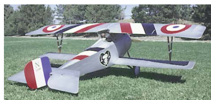
CD042 NIEUPORT 17. Here's the "right size" sport scale R/C model of the WWI fighter. At 68-inch span, this 1/2 scale model is IMAA legal, but still easily transported, and needs only a .53-.65 4-stroke engine. Plans on two sheets. Pat Tirtle. FM 12-97. $$$
