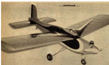
CF021 SKYLINER. Shoulder wing, 4 to 5 channel design, with 60 inch span, for great R/C sport flying. M. Meyer. FM 8-65. $$J
