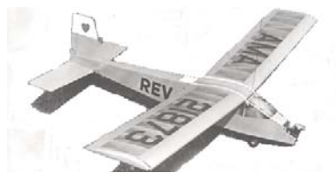
CF415 REVISION A. Single or 2 channel R/C trainer, featuring 44-inch span. For .09 eng. H. Applegate. FM 8-76. $$$C
