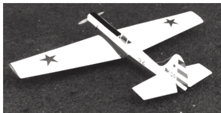
CF810 YAK-50. Aerobatic 60-inch span R/C sport-scale design for 25 size electric motors. 4 channel radio. B. Bowne FM 9-89. $$F
