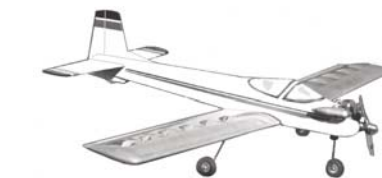
CF642 PEPPER. Low wing R/C sport design with 50-inch span. .19 to .25 eng., 4 channel R/C. D. Sarpolus. FM 9-83. $$D
