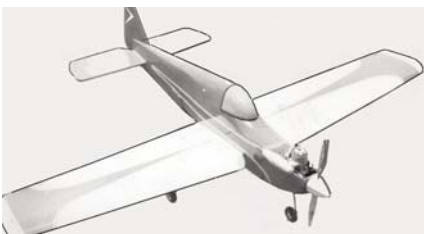
CF640 SPINNER II. Sleek R/C pattern-trainer for .60 eng., and 4 channel gear. Features 63-inch span. Foam and balsa construction. M. Blackard. FM 8-83. $$D
