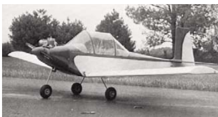
CF739 JEA S-1. Four-times "Peanut Scale" size R/C model of Japanese homebuilt lightplane. Uses .25 to .40 eng., 4 channel guidance. T. Houle. FM 1-87. $$$J
