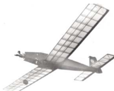
CF655 PONG TWO. Low-wing 1/2A sport ship, 2 channel gear, built-up construction, 44-inch span. L. F. Randolph. FM 2-84. $$C
