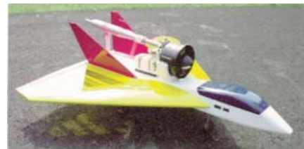
CD175 SUNSPOT A kit bash of the popular delta pusher, the Force One , designed by Laddie Mikulasko and kitted by Balsa USA. This revision utilizes fan power from a K&B 7.5DF and Turbax I fan system. A stretched nose and larger fins streamline the model. Wing spans 36½ inches. Finished weight is 6 pounds. Single sheet plan shows only changes to the stock kit. Wallace Louie. FM 08-2002 $$$D
