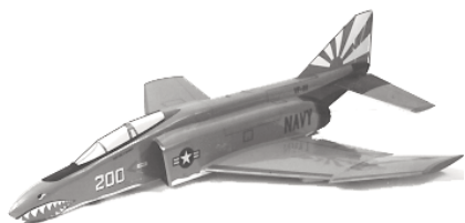
CF757 PERFORMANCE PHANTOM. An R/C, ducted fan hot rod. Balsa and foam construction. Uses Dynamax or Turbax fan, and .60 to .80 eng. Requires 4 to 5 channel gear. Plans on 2 sheets. E. Baugher. FM 9-87. $$$Q
