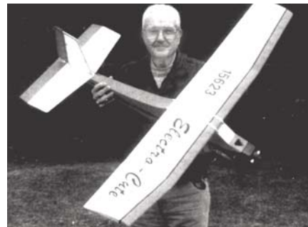
CD018 ELECTRO-CUTE. If you want to try your hand at electric R/C, this 4-channel ship offers the economy of 05 power in a pleasant flying high wing model. Spans 55 inches and is 41 inches long. Bill Passarelli. FM 3-97. $$$D
