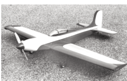
CF540 VIRGINIA SLIM. R/C Sport-Pattern design has molded plywood fuselage, 56-inch span, .60 eng., 4 channel guidance. D. Reiss. FM 6-80. $$$D
