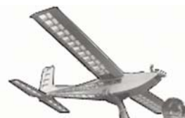
CF282 TYCHO 400. Altimeter equipped R/C trainer for .45 eng., 4 channel R/C units, 62-inch span. D. McGovern. FM 12-72. $$$
