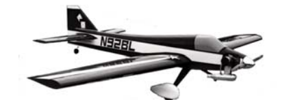
CF619 GAMBLER. R/C Sport-Pattern design with 700 sq. inch wing and .60 power. Has scale like looks. B. Lobozzo. FM 1-83. $$D
