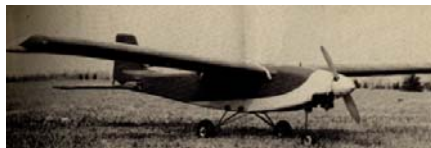
CF005 CITATION. Multi channel R/C design for .35 to .45 eng. High wing model has 63-inch span, Roth. FM 8-62. $$J
