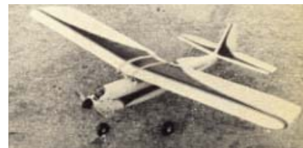
CF054 KOBRA II. Sporty shoulder-wing, tri-cycle gear design which features a high tail placement and 60-inch span. It takes .29 to .35 eng. G. Rogers. FM 10-66. $$D
