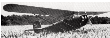
CF623 AMERICAN EAGLE EAGLET. 1930s design, R/C Stand-Off Scale features big 68-inch span and .35 power. For 3 to 4 channel gear. A. Wolsky. FM 2-83. $$D
