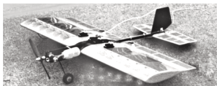
CF909 LITTLE FUN. Easy to build 1/2A Fun-Fly design for 4 channel or mixing radio systems. 27-inch spans, uses an .049 to .051 eng. D. Sarpolus FM 7-93. $$B
