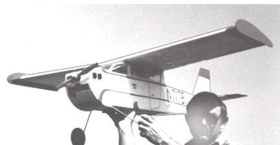
CF733 LACEY M-10. Easy-to-build R/C sport-scale design, 55-inch span, 4 channel R/C,.35-.40 eng. D. Snull. FM 10-86. $$Q
