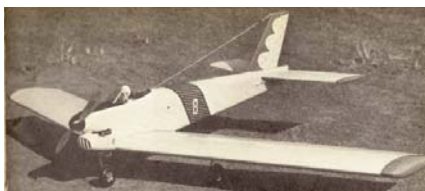
CF032 MARK 8. Aerobatic R/C sportster for 4 to 5 channel and .60 eng. 67-inch span, built-up, swept wing and tri-cycle landing gear. P. Foster. FM 4-66. $$D
