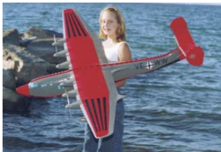
CD091 POTEZ-CAMS 161. Designed for six Speed 400 motors, powered by two 10-cell 1700 mAh batteries. Construction is mostly foam, with some balsa. It qualifies as IMAA legal at 80-inch span. The 3-sheet plan includes all templates, motor and battery circuit, and a detailed isometric. Laddie Mikulasko. FM 8-99. $$R
