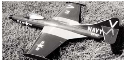
CD108 F9F PANTHER. This jet uses a cobalt 05 motor driving an APC 7-7 prop. Spans 39 1/4 inches, and needs a 3-channel radio. Can also use a brushless motor. Pat Trittle. FM 04-2000. $$D
