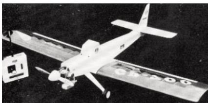
CF527 GP 700. General purpose airplane for glider tow, featuring 60-inch span, .60 eng., 4 channel units. B. Aberle. FM 1-80. $$$D
