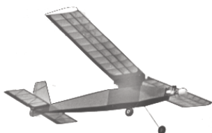
CF569 PONG. 44-inch span R/C model for .049 eng. 2 channel radio. Designed for small field flying. L. F. Randolph. FM 5-81. $$C
