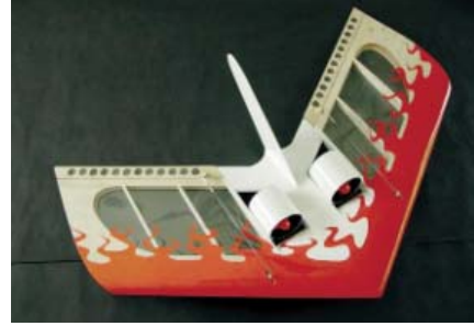
CD217 JET JUNIOR An R/C twin electric ducted fan sport model suitable for park flying. All balsa construction with a wing span of 26¼ inches. Weight is 11 ounces. For three channels, it uses EDF-50 fans. Plans on one sheet. Olan Hanley. FM 03-2004 $$$C
