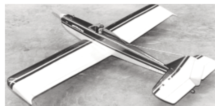
CD008 VOLTMASTER. Sizable electric R/C ship has performance and duration. All balsa with novel powertrain pull-out tray. Spans 69 inches, for 21 cells, ModelairTech H-1000 belt drive. Gene Rogers. FM 11-96. $$$D
