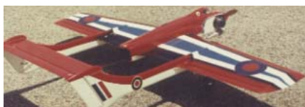
CF281 SEA VIXEN. 64-inch span R/C sport-pattern twin boom design uses 4 channel R/C gear, .60 eng. J. Sheeks. FM 11-72. $$$
