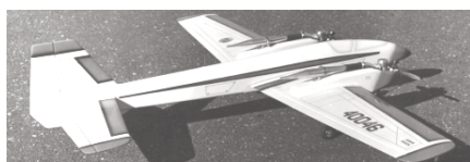
CF483 MAGNUM 80. Fast and powerful R/C Sport-Pattern twin for .40 engs. Features 76-inch span, and uses 4 channel gear. D. Sarpolus. FM 9-78. $$$D
