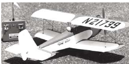
CF426 WREN. R/C sport-biplane requires .15 to .19 eng., 38-inch span. For 4 channel gear. N. Rosenstock. FM 12-76. $$$D
