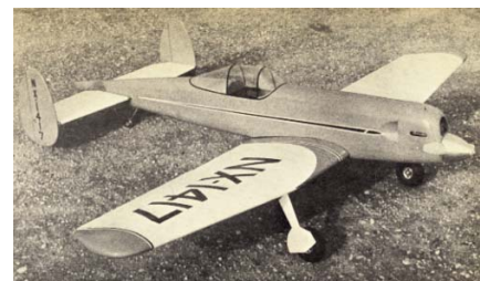
CF072 DEFENDER. Parasol wing, 65-inch span design with removable tray for 4 channel R/C gear. Takes .45 eng. G. Rogers. FM 4-67. $$D
