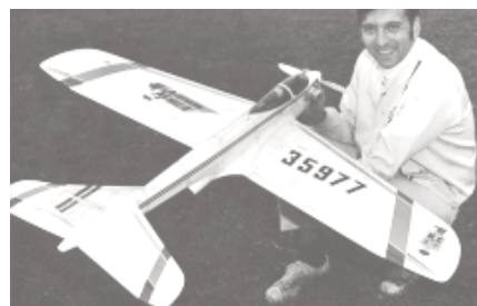
CF310 NORTHERN EAGLE. R/C Sport-Pattern, 58-inch span, .40 to .51 eng., 4 to 5 channel R/C. D. Gierke. FM 9-73. $$$
