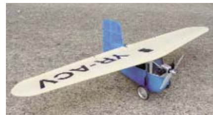
CD223 STABILOPLAN IV A R/C semi-scale electric powered homebuilt aircraft. It's basically a flying wing with a big trunk, and as the name implies, it is very stable in flight. Light weight balsa construction, it can be powered with a brushed or brushless motor system. For three channel control. Its wing spans 44 1/4 inches. Weight is 15.1 ounces. Plans on one sheet. Dick Miller. FM 05-2004 $$C
