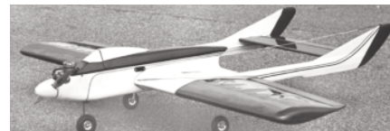
CF550 VAMP. R/C Sport-Pattern, twin-boom ship with 58-inch span, .40 eng., and 4 channel gear. J. Sheeks. FM 10-80. $$$D
