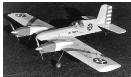
CF967 DOUBLE IMPACT. Twin engine sport R/C aerobatic design. 74-inch span, 4 channel, two .40 to .51 engines. Dick Sarpolus. FM 7-95. $$G
