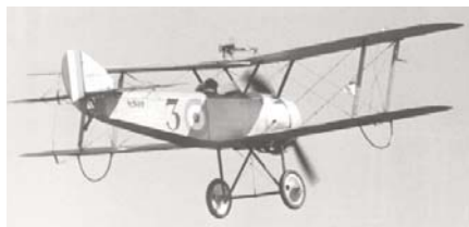
CF391 SOPWITH PUP. WWI Stand-Off Scale R/C with 59-inch span, .60 eng., 4 channel system. J. Puleo. FM 12-75. $$F
