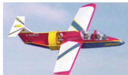
CD141 RFB600 FANTRAINER An R/C Sport Scale ducted fan, without the ducting. All balsawood construction, except for the wing which has a foam core. With a wing span of 77 inches, its finished weight is about 11½ pounds with optional retracts. Requires a .61 to .75 engine, and 4-6 channel radio gear. Canopy and servo fairing available from the author. Greg Moore. FM 07-2001 $$$Q
