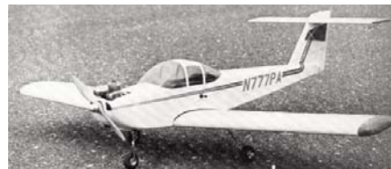
CF520 PIPER TOMAHAWK. R/C Stand-Off Scale model of popular private trainer for .19 to .30 eng., and 4 channel gear. Has 50-inch span. D. Sarpolus. FM 10-79. $$D
