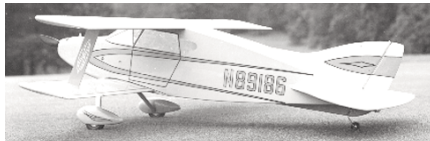
CF349 HIPERBIPE. Wild looking R/C Stand-Off Scale biplane, 45-inch span, 4 channel R/C, .40 eng. S. Hines. FM 11-74. $$$D
