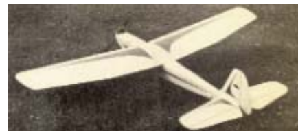
CF042 LUCKY 2. Fine flying, 4 channel R/C shoulder-wing design with 60-inch span. For .45 eng. G. Rogers. FM 7-66. $$D
