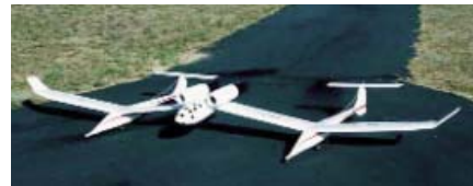
CD210 WHITE KNIGHT Join the next 100 years of flight with this electric ducted fan scale model of Burt Rutan's futuristic launch aircraft for space flight. An R/C giant, its wing spans 134 inches and has an area of 1044 square inches. Power required are two Midi Fans with Mega 22/30/3 motors on two 30-cell packs. Construction is balsa over foam for the wings, balsa and ply for the booms, and fiberglass for the pod and nacelles. Finished weight 16 pounds. Plans on four sheets. Ivan Munninghoff. FM 12-2003 $$$U
