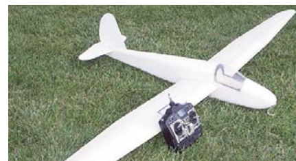
CD305 SCHWEIZER 1-23 STANDARD. An R/C scale glider, constructed of expanded polypropylene foam and sheet balsa. This plane has an SD 7037 airfoil, with a 57 1/2-inch wing span, wing area of 587 square inches, length of 57 1/2 inches and weighs 48 ounces, that gives this glider a wing loading of 13 ounces per square foot. Plans on two sheets. Thomas J. Martin. FM 03-2007 $$$L
