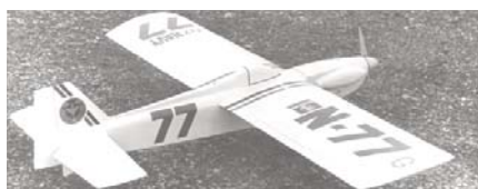
CF216 DEE-KAY SPECIAL. Formula II R/C pylon racer with 57-inch span, hot .40 eng., 4 channel gear. D. Gierke. FM 6-71. $$D
