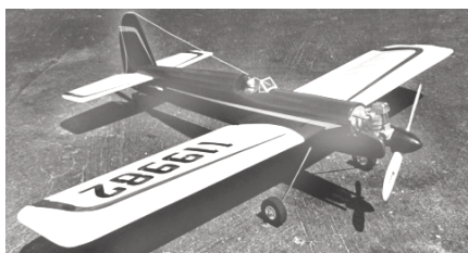
CF777 FOUR PLAY. Just the ticket for .20 size 4-stroke eng. Spans 47 inches, 4 channel R/C system. D. Sarpolus. FM 6-88. $$C
