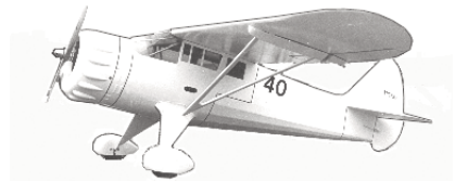
CF510 MR MULLIGAN. 1930's classic racer makes great R/C Stand-Off Scale model with 67-inch span. Requires .60 eng., and 4 channel R/C system. T. Lombardo and D. Palumbo. FM 7-79. $$F
