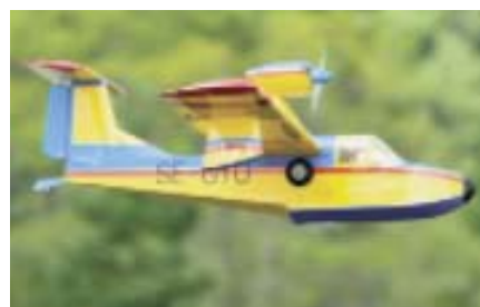
CD349 THURSTON TEAL. Beautiful 70-inch R/C amphibian perfectly suited for electric power, but .40 size glow can be substituted. Has manually retractable landing gear for wet or dry runways. Traditional balsa and ply construction. Plans on three sheets. Laddie Mikulasko. FM 08-2008 $$U
