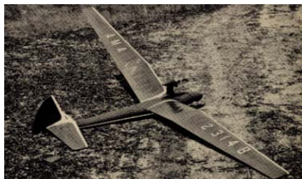
CF014 SEAGULL. Giant 101" span R/C soarer with supplementary .09 to .15 power. D. McGovern. FM 8-62. $$J
