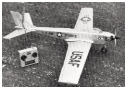
CF261 ASTEROID. Unusual looking R/C sport design with 61-inch span. For 4 channel radios, .40 eng. D. Johnson. FM 4-72. $$$
