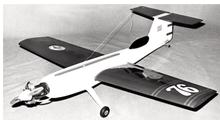
CF405 76 SPECIAL. Quarter midget R/C trainer with T tail, for .15 eng. Has 36-inch span B. Aberle. FM 5-76. $$$D
