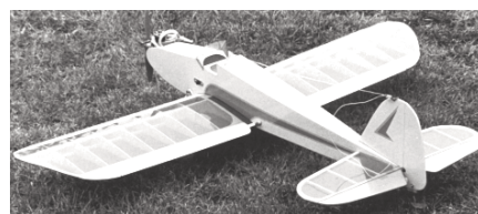
CF793 GEE-HAW. Sporty low-wing design for G-Mark .061 or similar eng., and 4 channel micro radio systems. Spans 37 inches. L.F. Randolph. FM 2-89. $$C
