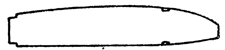
TAILPLANE RIB NO. 1 MAKE 2 FROM \frac{1}{8} " Balsa SHEET
