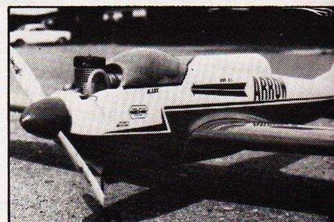
Super Tigre X 60 proved to be good power choice for this project; note pipe setup.
