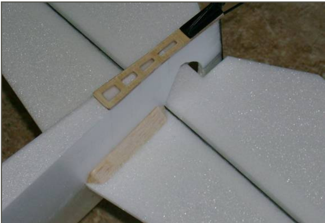
Figure 16 - Horizontal Stabilizer Balsa Doubler Detail
