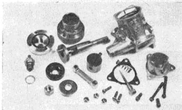
Component parts of the "Pet" showing the revised cylinder design.
