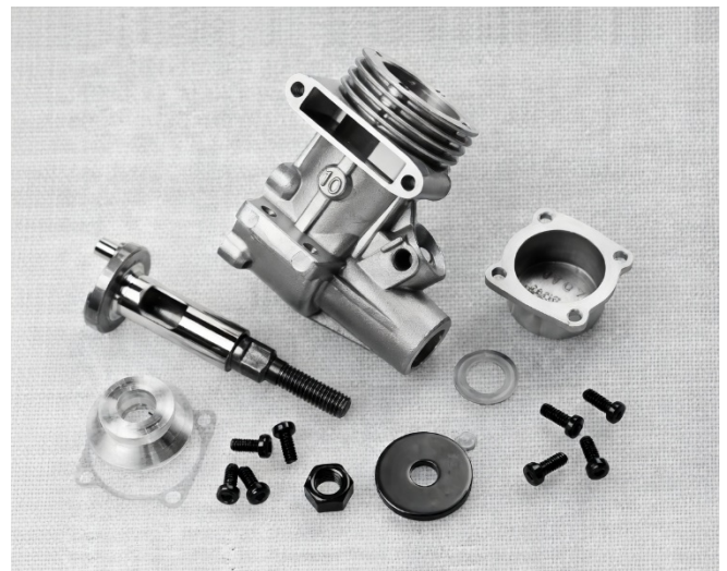
Neat pressure cast crankcase includes wide exhaust stack which conducts gas from exhaust port in rear right quarter of the liner.
