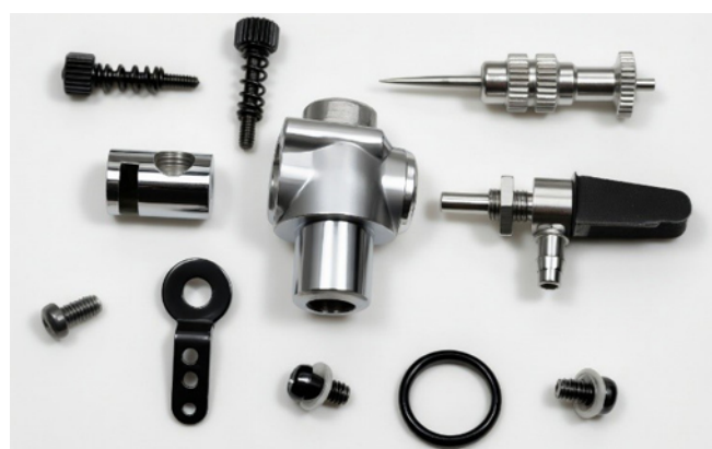
Bottom right: parts of the latest throttle type carburettor fitted to the Max-III-15R/C.
