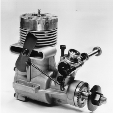
Below, one of the bolter .35 cu in. radio control engines, the O.S. Max- H.35 R/C
