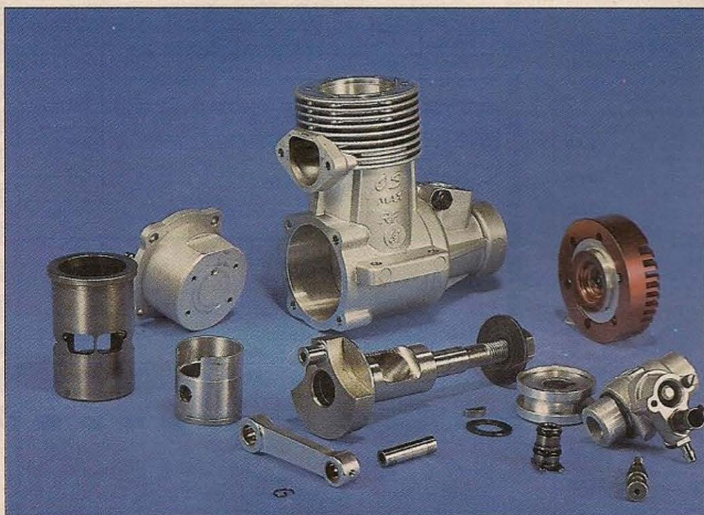
No one beats O.S. when it comes to design and craftsmanship. The .61RF features an ABC piston/cylinder, a massive 17mm crankshaft journal and an aluminum bar stock conrod with bushings at both ends.
