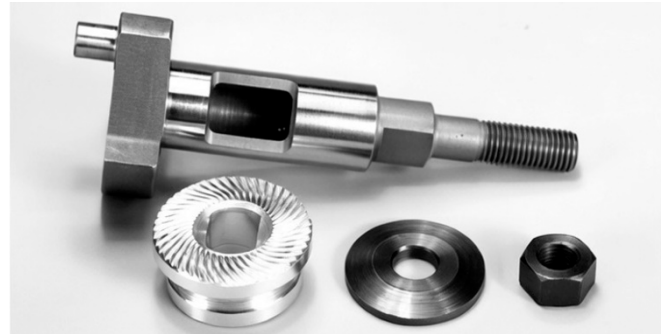
Crankshaft and prop drive washers and nut. Note massive width of counterbalance. Prop drive washer is driven by flats on crankshaft rather than a collet or key. 5/16"-24 prop threads used.
