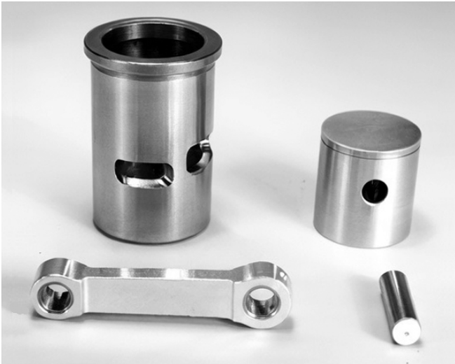
Piston, sleeve, rod, and wrist pin assembly. Even though an economy engine, the rod is bronze bushed at both the crank pin and wrist pin ends.
