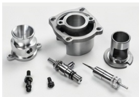
Rear induction assembly showing drum type rotary valve. 10 mm. racing venturi, angled needle assy.
