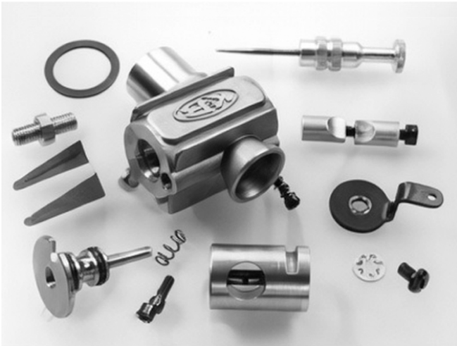
Parts of the K&B automix carb. Mixture control valve (left, foreground) is adjusted by means of adjacent eccentric headed screw.
