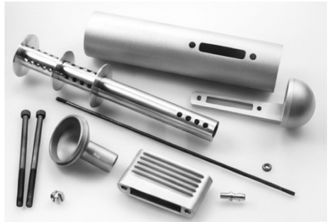
Muffler parts. Perforated central tube with baffles provides better noise suppression than conventional expansion chamber.
