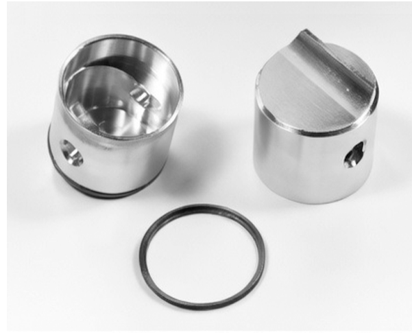
Prominent design feature is aluminum piston with special single L section ring.
