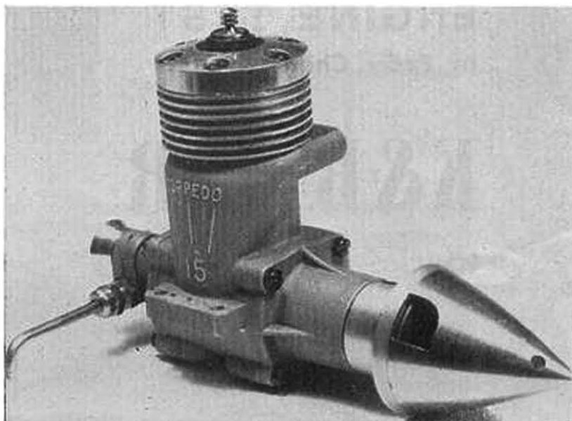
Three-quarter front view of the Torpedo .15R, shows bolt on front housing and peripheral six jet carburettor mounted on backplate. Note the unfinned cylinder head and large transfer passage.
