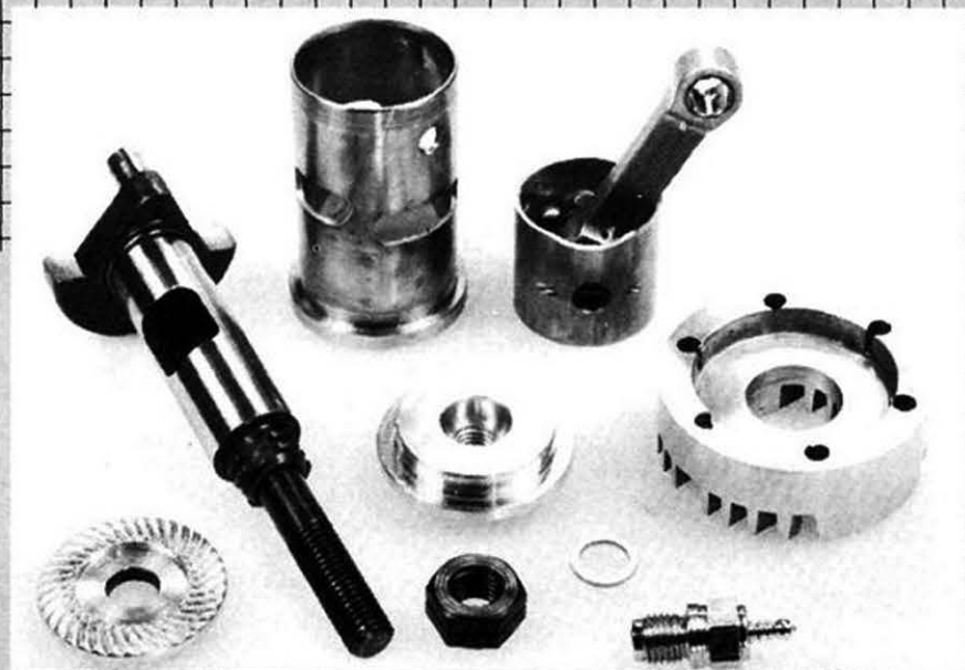
"Series 6" has switched to ABC piston/liner construction. Note unorthodox method of retaining wristpin with small roll pin through piston.
