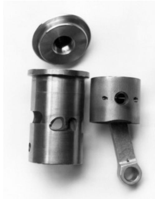
Front view of piston/cylinder shows inclined Schnuerle ports through cylinder wall and also the unique method of retaining the wrist pin inside the piston with a tiny steel roll pin.
