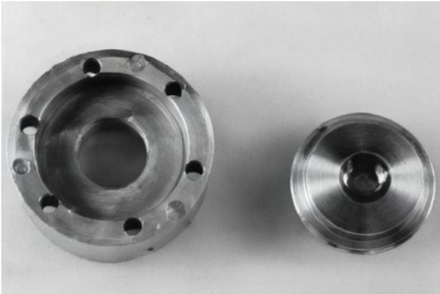
Two piece head assembly. Head button very wide eguish area surrounding small combustion chamber bowl.
