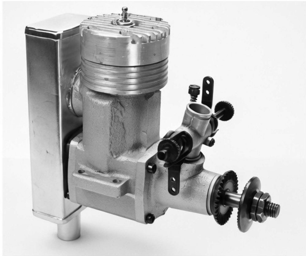
Fox 36RX is a new kind of power package for the sport flier. Muffler is designed to fit between engine bearers and inside cowl; engine uses sand castings.
