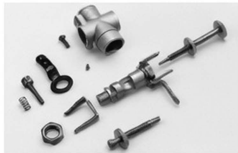
Carb features separate high- and low-speed jets, individually adjustable.
