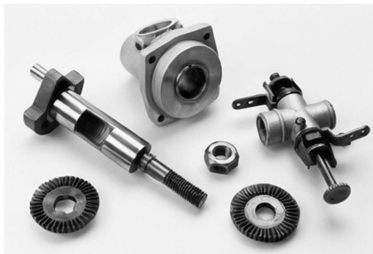
Crankshaft runs in a bronze main bearing. Front housing, like main casting and backplate, is a sand casting.
