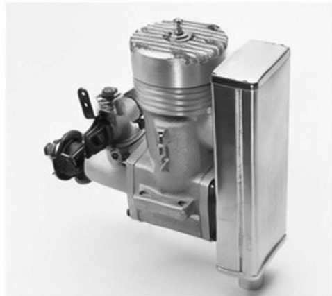
With in-cowl muffler, increased flow of cooling air is needed.
