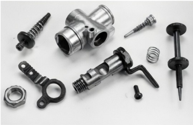
New carburetor parts: separate high/low speed jets have own adjustment.
