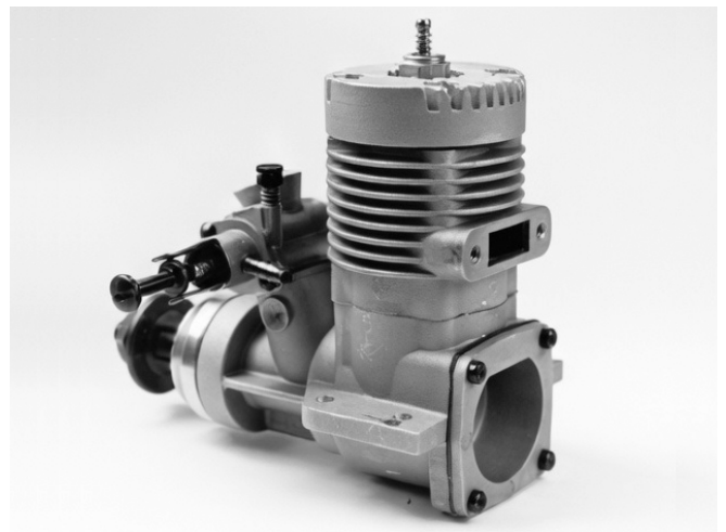
Above right feature of Fox 19 BB is a separate cylinder jacket and 90 transfer channel enabling exhaust to be rotated to rear or either side.
