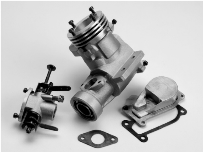
New 15 resembles current Fox 40/45 series in layout with usual crankcase and back plate.
