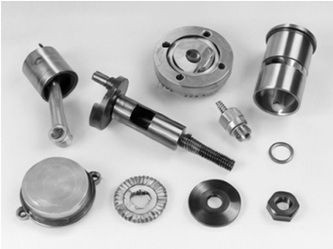
Fox 15 uses traditional crossflow porting with lapped cast-iron piston running in steel cylinder sleeve.
