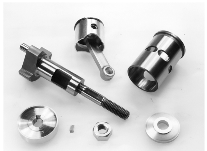
Crankshaft and piston/cylinder components of the Super Sport 30-RING. Note sturdy crankshaft and quality finish.
