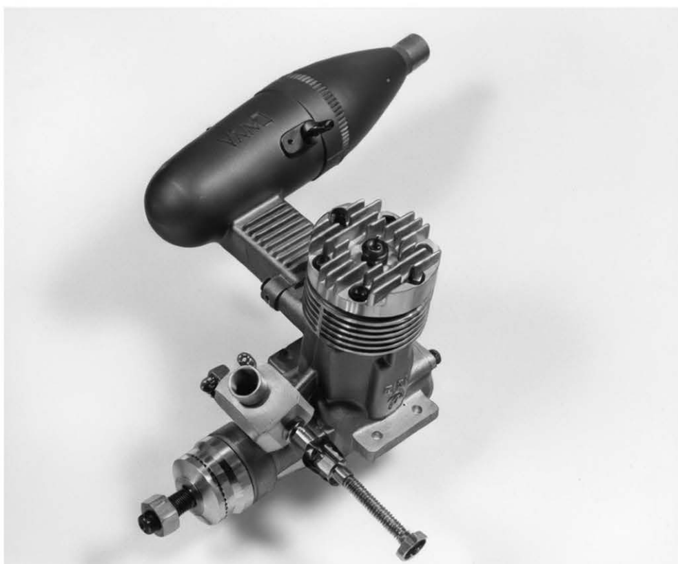
Enya 49X broken down into its component parts (above). Note porting of sleeve at center of photo. Polished head and streamlined muffler makes for an attractive engine (below). Carb bore just visible.
