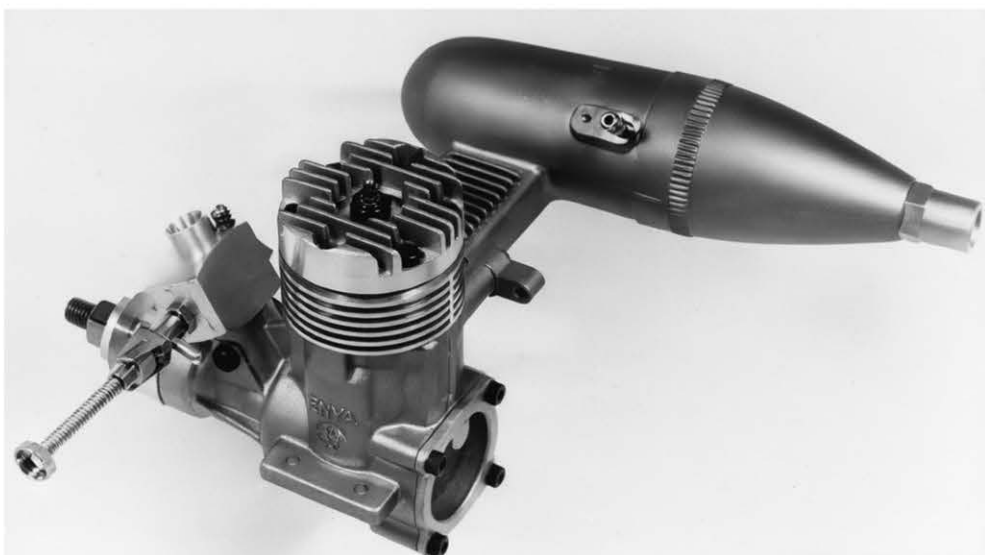
Enya 49X shown with silencer. The muffler is fitted with pressure tap for use in pressurized fuel systems. Note spring type needle valve which allows settings to be made away from prop arc. Four bolt rear plate.
