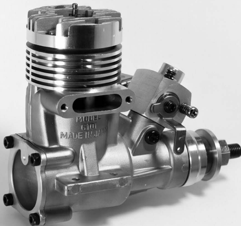
The 49X is typical of the kind of craftsmanship for which Enya is well known. This new motor features a ringed piston with a steel liner. The carburetor is the standard machined aluminum Enya model.
