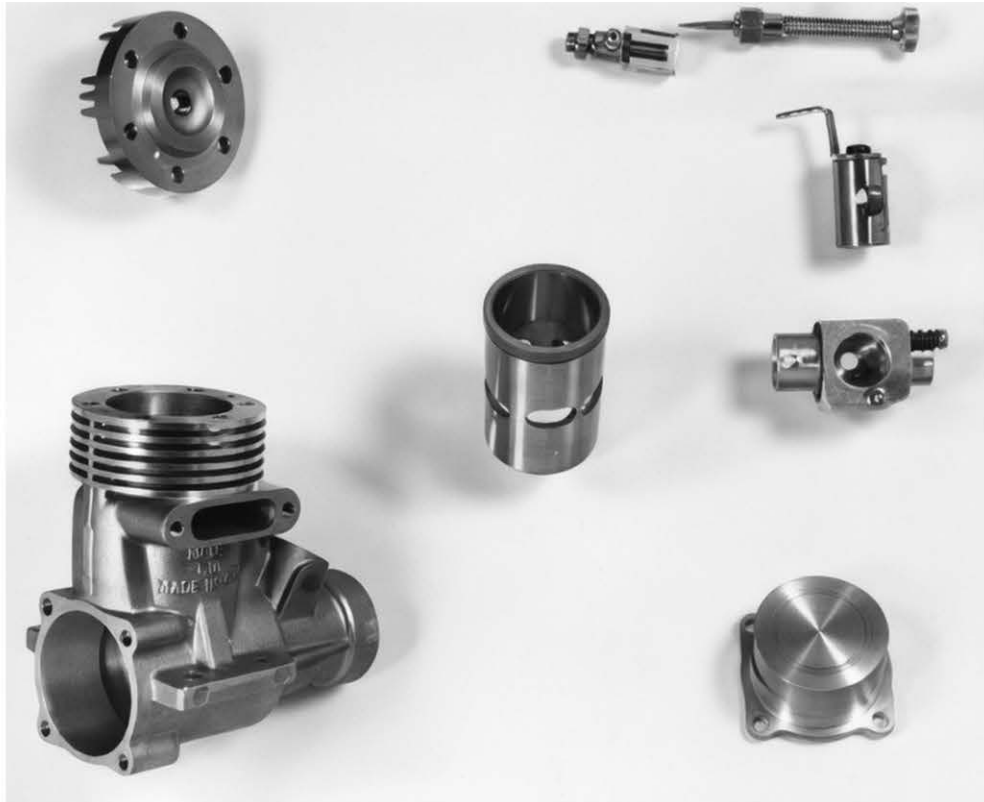
Enya 49X broken down into its component parts (above). Note porting of sleeve at center of photo. Polished head and streamlined muffler makes for an attractive engine (below). Carb bore just visible.
