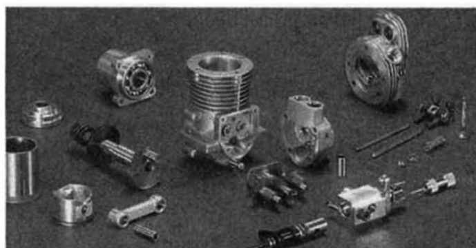
The rear main ball bearing acts as "locator" into crankcase. The piston and front housing have been machined out of solid aluminum alloy. The cam drive and cams have been hardened.
