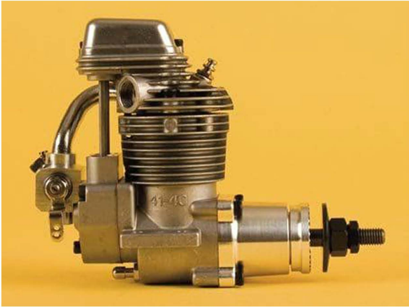
Here, the air-bleed idler hole is at rear of the carb. This relatively small 4-stroke muffler just meets regulation noise levels.
