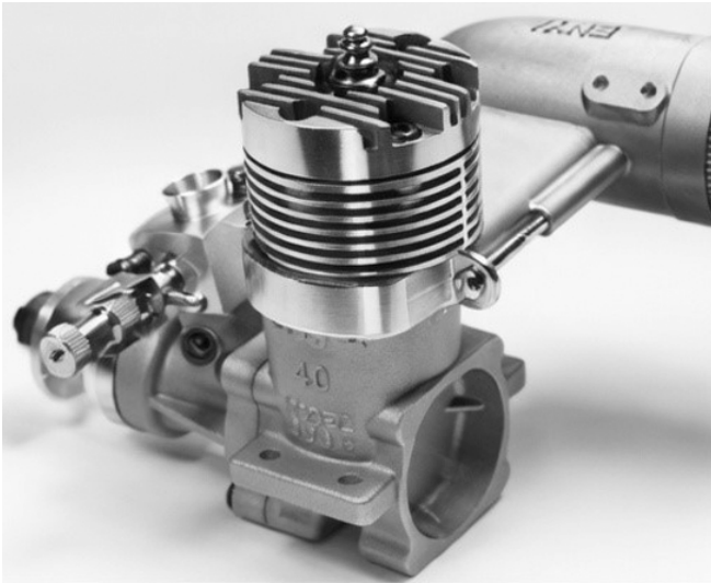
The motor is shown at left without silencer and above with Enya M-200 type. Note strap fixing and substantial lugs on silencer casting.
