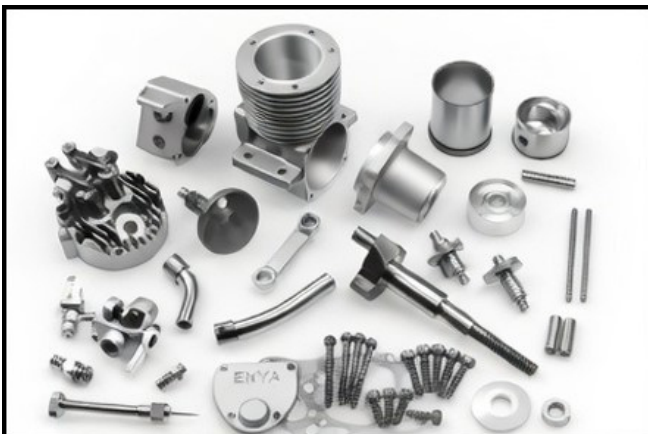
Below left: basically a larger bore version of the Enya 35-4C the 40-4C also differs from its smaller brother in having a ringed piston running in a steel cylinder liner instead of a ringless piston in a chromed aluminum liner.
