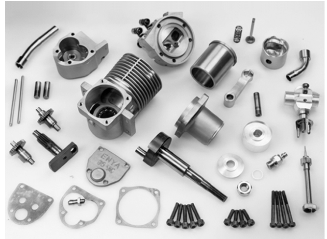
Right: Parts of the Enya 35-4C. Engine features twin camshafts and has a ringless aluminum piston running in a chromed aluminum liner.
