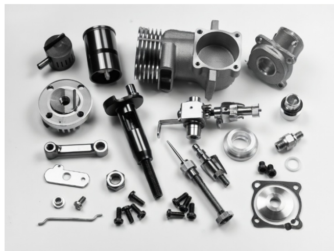
Parts of the 19-V, including TV carburetor. New version has bigger bore, shorter stroke.
