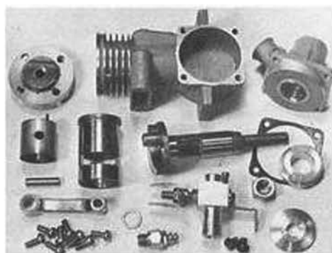
Parts are sturdy and well-finished. Engine can be converted to opposite rotation by repositioning the front housing at 90 degrees.
