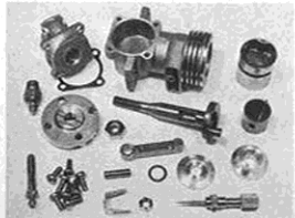
Parts show good finish and machining throughout. Note thick liner with bypass flutes.
