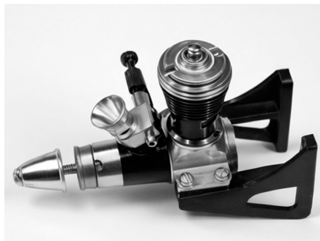
Moulded engine mounts, made by L. M. Cox for the Tee Dee .049 convert it to a firewall radial mounting as seen in above view.
