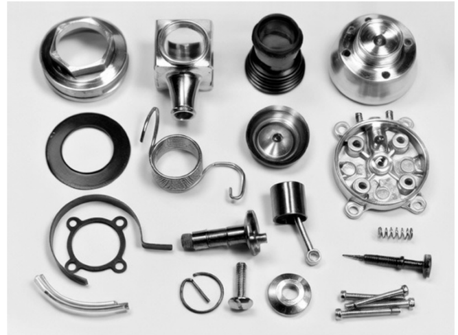
Functional, lightweight parts of the .049 QZ laid out for inspection.
