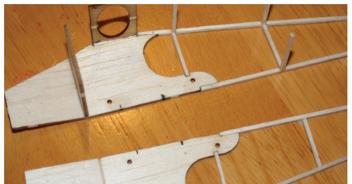
UC F2 and some cross braces added to one side. Note the score mark where the sides crack in to the nose.
