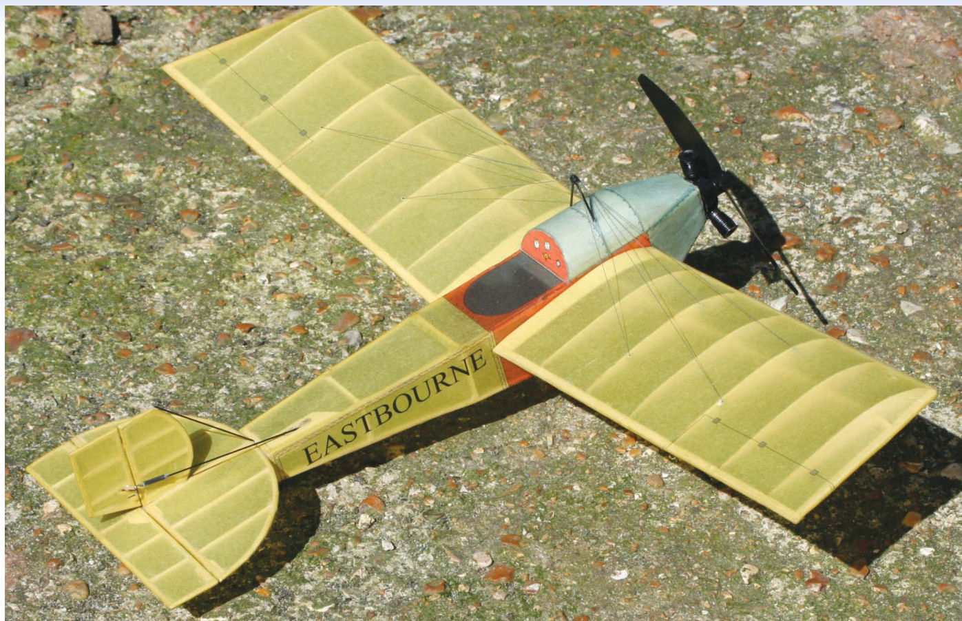
The concrete lends scale to the model. This shot clearly shows the reinforcing at the wing root and the buckled rib on the far wing.
