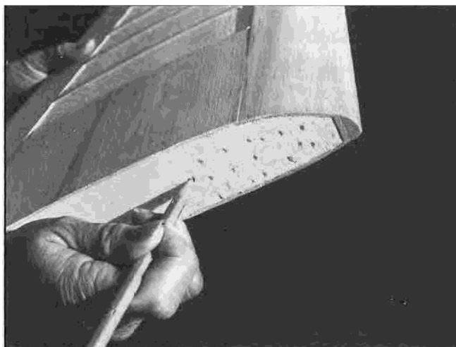
Prior to joining wing panels, puncture root of cores with pencil to give epoxy more grasp.
