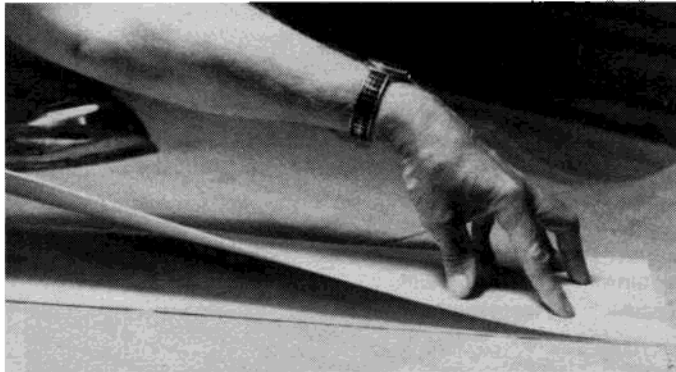
LEFT: The two pieces for the boom with grain running the same way, put web between and iron same way. RIGHT: Iron both sides until very hot, wood may turn brown, then cool.
