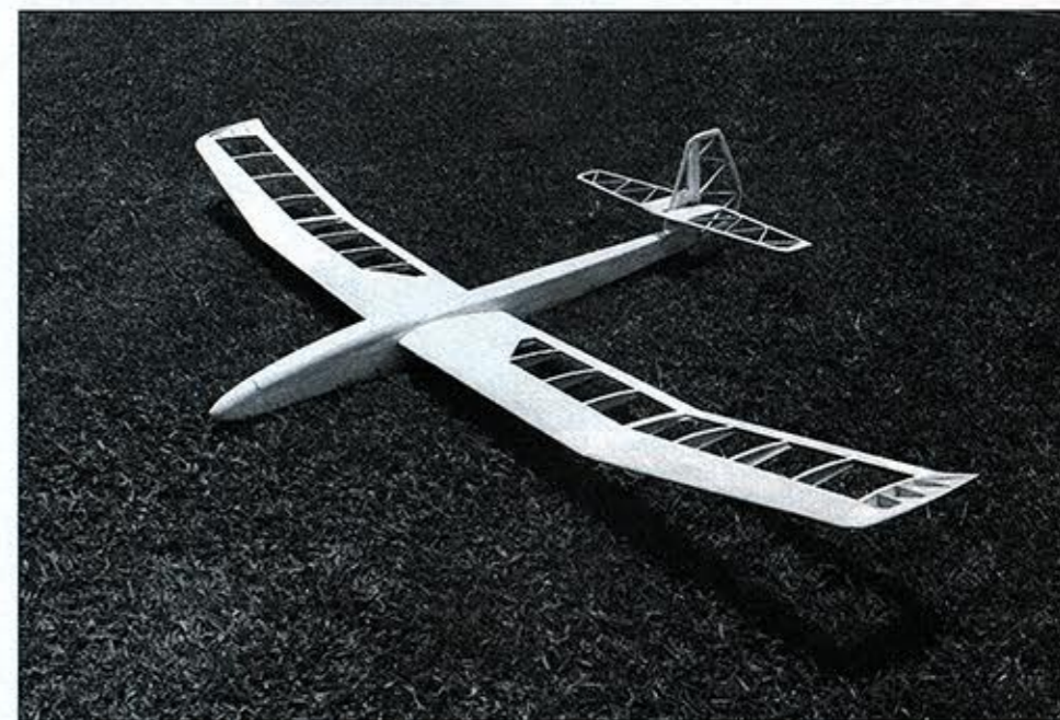
Structure detail. Note the built-up wing tips.
