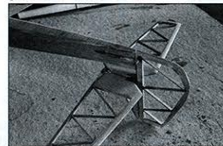
Rudder and stabilator control hook up.
