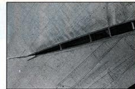
Routing of the stabilator and rudder sheathing. Note that the yellow rods are inserted to prevent buckling of red sheathing.
