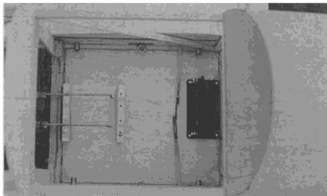
No shortage of radio mounting room in the Wimpy! Note the 1/4-inch tubes that locate wing to fuse, also hooks for rubber bands.
