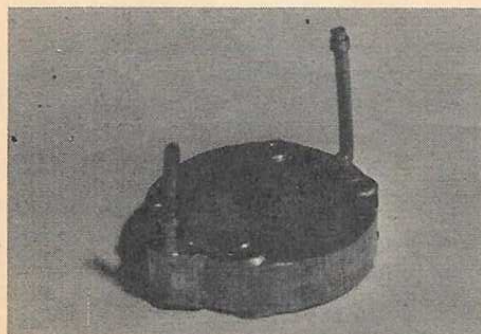
This is the tank for Cox Tee-Dee, it works fine.
