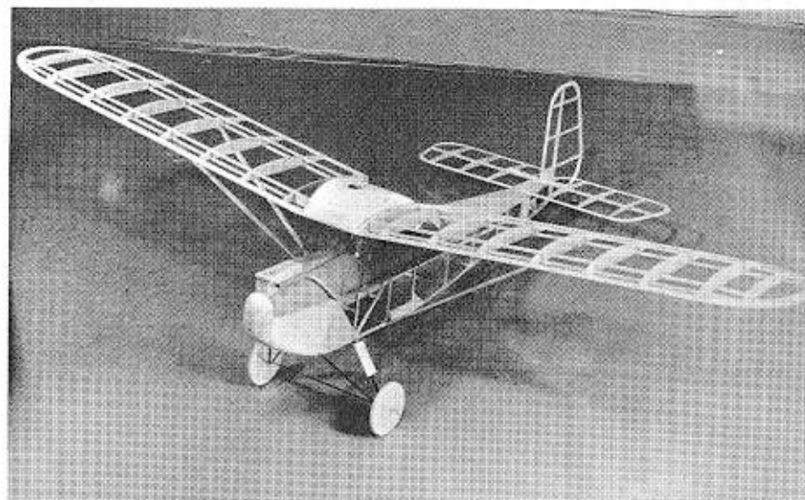
This shot of the uncovered Widgeon gives some idea of the structural detail and assembly.
