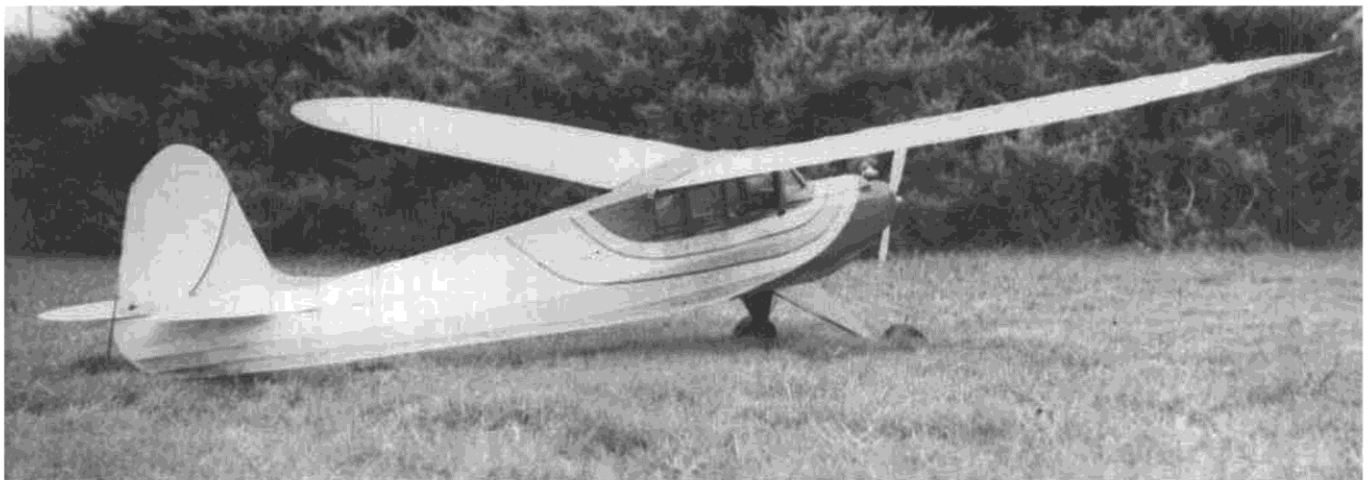
May seem a bit large for an .049 engine, but the West'ner is really nothing more than a powered glider. The Ace Pulse Commander system keeps the weight down, and also keeps the model in sight of the flier!
