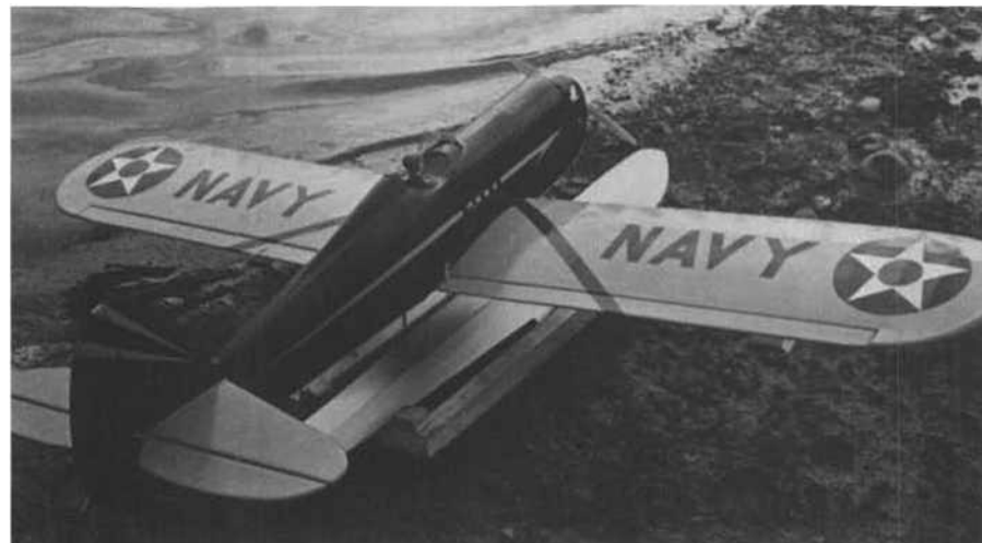
Water Strider is quite large and weighs ten pounds, yet the OS .60 has no trouble getting it off the water. Properly designed seaplanes don't need tons of horsepower to get "unstuck."
