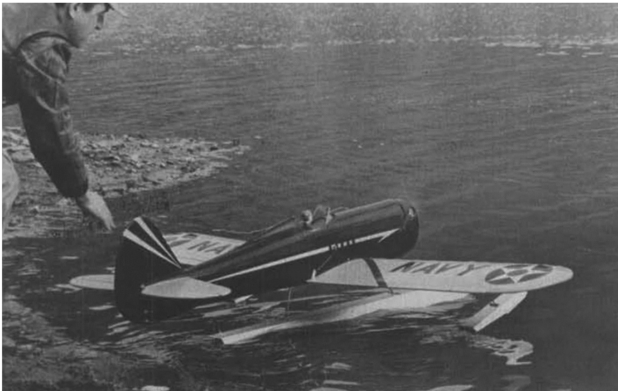
Bob von Koňsky launching his Water Strider. Tip floats just barely tick the water's surface and do a good job of keeping the wings straight during all water operations.
