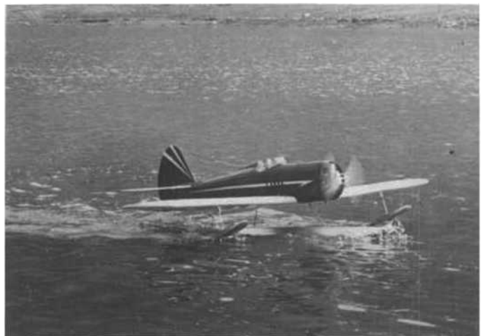
Handling characteristics of the single float are excellent. Tip floats are at such an angle that they cannot dig in, yet do their job.
