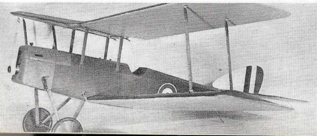
Left: dressed in R.F.C. markings the Warrior prepares for the dawn patrol. 42 in. span machine takes 1.5 c.c. motors and any of the popular single channel systems.
