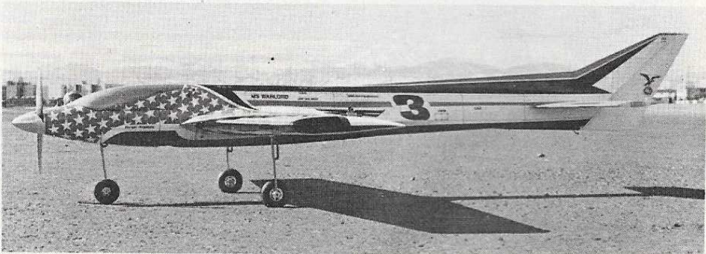
Top: Control surface areas are large; ailerons can be lowered for landing flaps. Note the highly recommended stall strip on the wing near the fuselage. Above: Heavily contoured fuselage is such that power can be utilized efficiently. Opposite, top: The wheel, when retracted, is partially out in the breeze; a big fuel tank fits easily. Bottom: There's a lot of room in front even with retracts.
