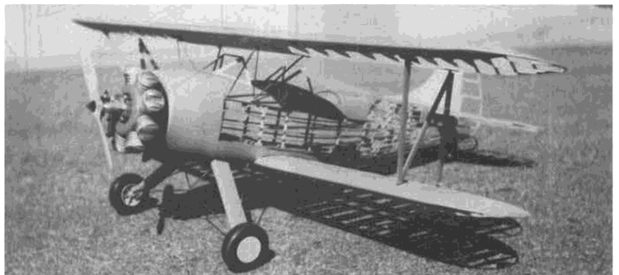
Framework shot of the author's model UPF-7. Plans were developed from Paul Matt 3-views, published in his Historical Aviation Album series.
