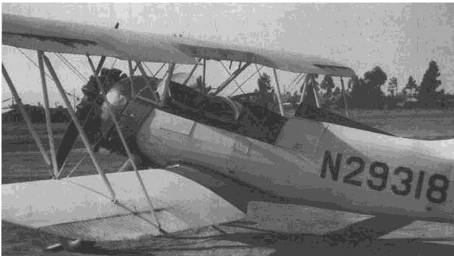
According to the registration number, this was only the 10th of 509 stock UPF-7s built. Note Waco insignia along side of cockpits. Top wing center section holds 50 gallons of fuel.
