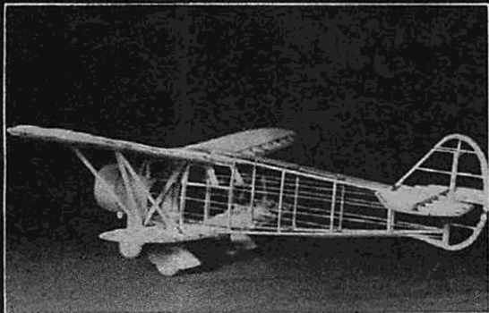
How the model is built. Note the simple, practical construction. Framework is very similar to real ship.
