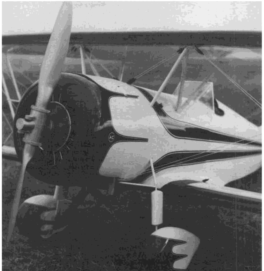
Larry certainly knows how to put on a nice finish! Fiberglass cowl and wheel parts are available from him, direct. See text. Dummy engine from Air Design.
