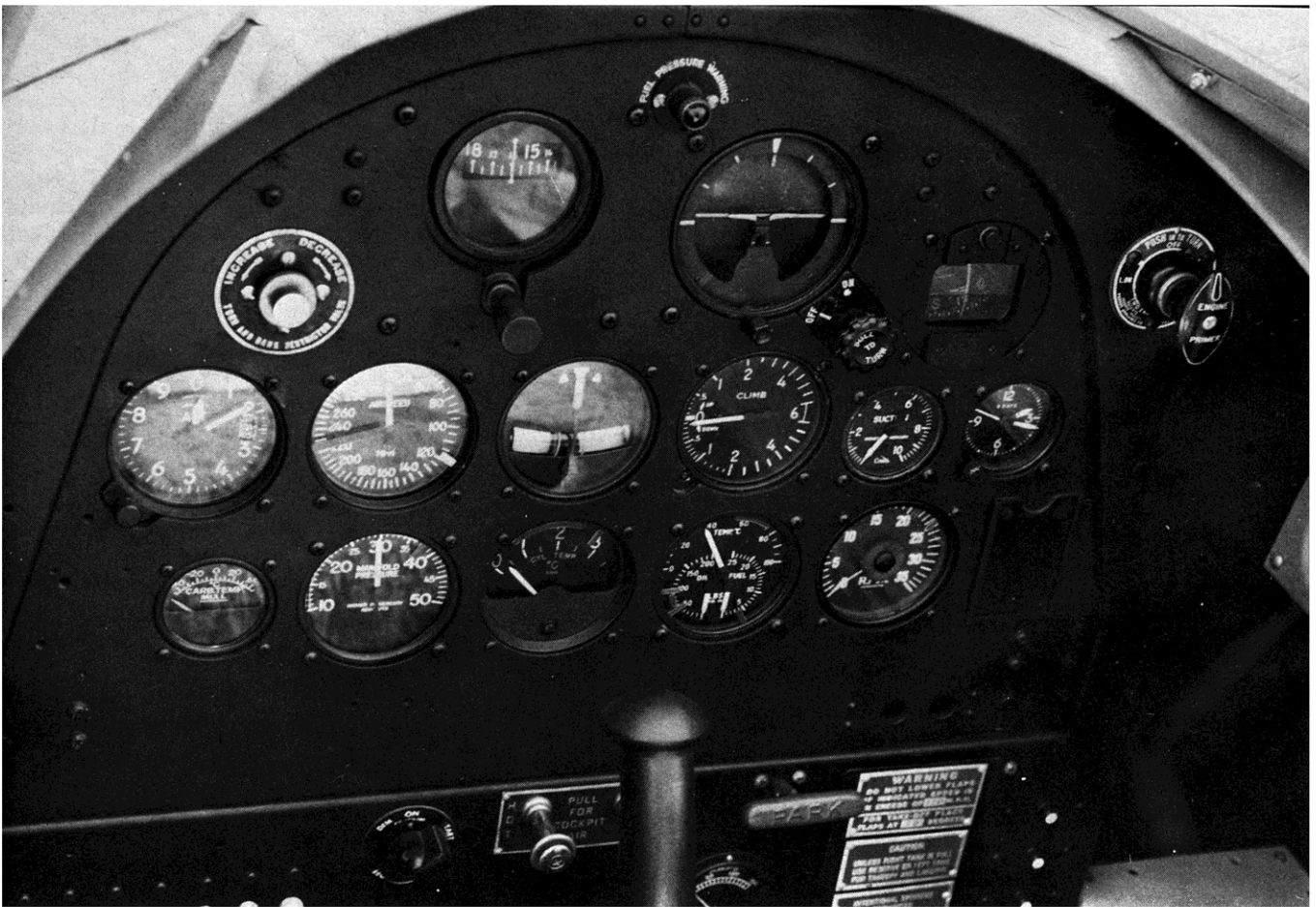
BT-13s were used to transition students from primary trainers to the low-wing fighter types. Simple instrument panel was sufficient for the job to be accomplished. Note airspeed red-line of 230 MPH, and flap-down of 120 MPH; also tumbled whiskey compass.
