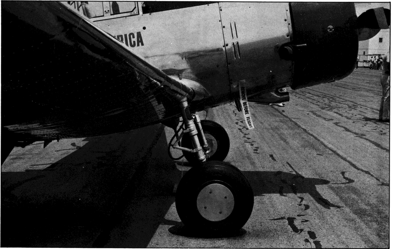
Stiff-legged BT-13 was made with a rugged landing gear to withstand the onslaught of the cadets' basic training.
