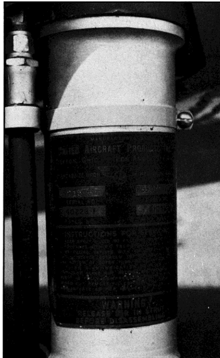
Closeup of manufacturer's plate on right gear strut. Line to the left is brake line.
