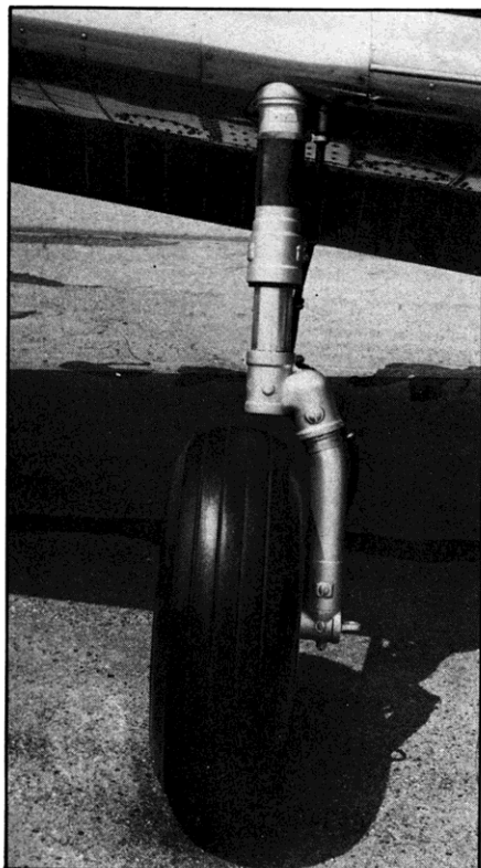
Strut is perpendicular to the ground, with a large amount of dihedral. The BT-13 was, and still is a very stable aircraft.
