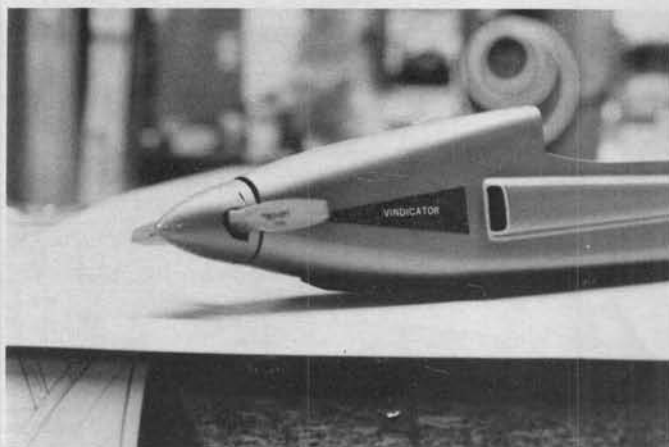
Airscops are fully functional. Be sure to cut away material as shown.
