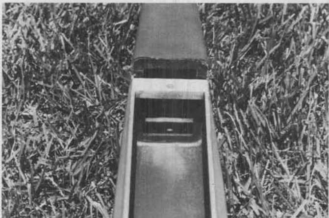
Primered fuselage, looking aft, showing detail of wing mounting block, and balsa wing saddles.
