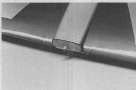
Completed wing with fairing and 1/4" hold-down dowel in place.
