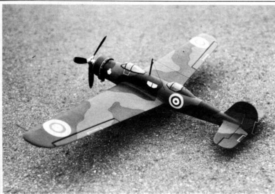
Left: The Tornado 3-bladed prop was painted dull black with silver tips and hub. Three-channel micro equipment operates throttle, ailerons, and elevator. Right: The 170 square-inch wing and 14-ounce all-up weight brings the wing loading to a light 12 oz/sq ft.
